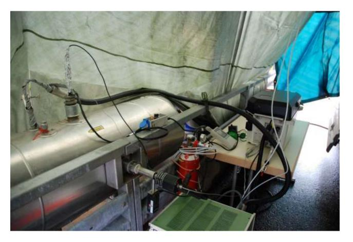
Heated sampling line to FID and humidity sensor because conversion to dry gas is needed
